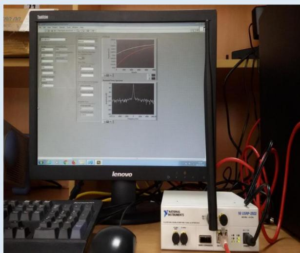
NI USRP Software defined radio platform interfaced with LabVIEW
